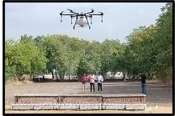
Fig. 2 : View of spraying of water by drone on the patternator.
